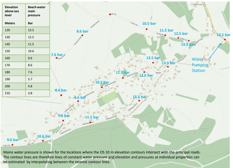
A column of water loses I atm (atmosphere) of pressure for each 10.33 m increase in vertical height, regardless of the pipe diameter, inclination, shape or flow rate.
